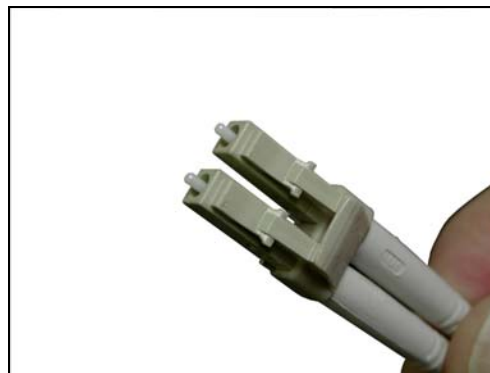
Figure 3-4 Fiber-optic Duplex LC Connector
